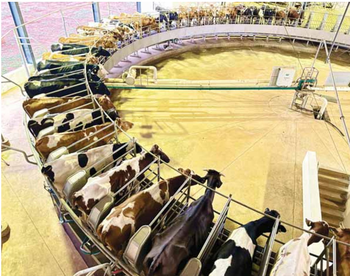
The dairy cows at the milking machine which entails teat cups, vacuum pumps, milk lines, milk receptacles, and systems for cleaning and sanitising the equipment.
